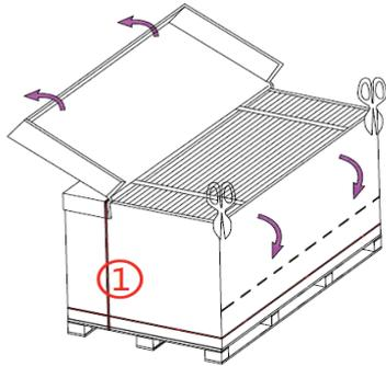
4. **Cutting the carton and fold it down**—Cut down the side of the carton by 1/2 to 2/3 height (keep at least 1/3 height), then cut down the side of the carton (the folding line is about the red line in the figure) and cut off the four packing straps inside the carton.
