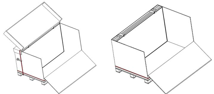
7. **Remove remaining modules**—Pour the remaining modules slowly, place them flat on the tray, and take out the remaining modules in turn.
