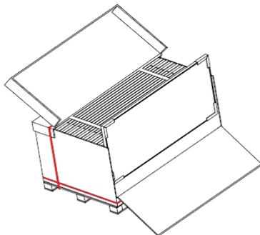
6. **Cutting the remaining packing straps**—When the remaining modules are covered by the uncut packing belt, two workers should hold the remaining modules, cut the no.1 packing belt and remove the top cover of the carton.
