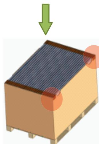
Remove the first module labeled "1" from the opening position (marked in red) firstly.
