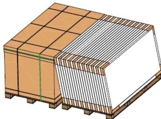
4. Two workers hold the modules to protect them from falling down. One of the workers cut the internal packing strap( totally 4 pieces of straps). The two workers then push the modules tenderly to lean them against the solid support and remove the modules from the first one outside to the last one inside in sequence.
