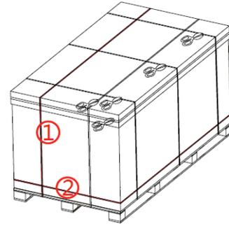
3. **Opening the box cover**—Open the box cover from that side where strap has been cut. Turn the cover over to no. 1 strap.
