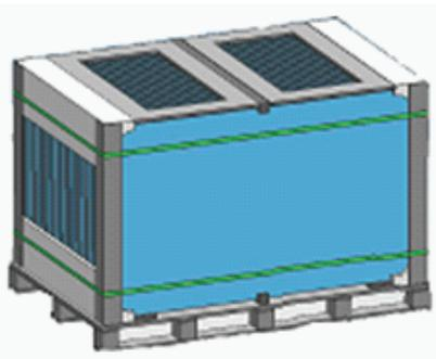
Cut off the whole packing belt of the pallet, and use a forklift to separate the two pallet modules.
