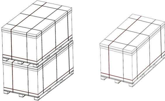
2. **Cutting packing straps**—Cutting all the packing tapes on the carton except no.1 strap and no.2 strap.
