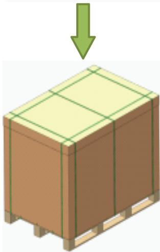
Cut off the packing tape of the single pallet, remove the isolated wood (or plastic wrap) and the carton cover.
