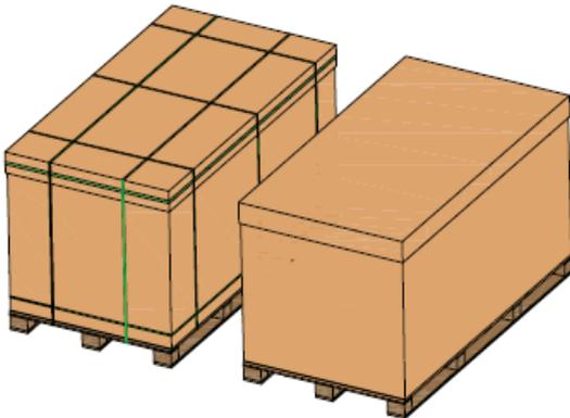
2. Leave the long side of the single box about 15~20 cm to solid support, such as wall, rack or unpacked module box of the same type. Then cut all the packing strap around the single box.
