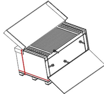
5. **Taking out the modules in turn**—Tear the tape from the first module border and remove the first module (make sure the remaining straps is tight to prevent the module from tipping). Tear off the tape on the frame in order of modules, and take out the remaining modules in order from the carton.
