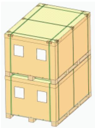
Cut off the whole packing belt of the pallet, and use a forklift to separate the two pallet modules.
